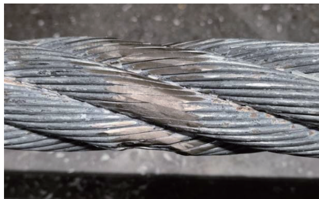
写真-3 断面欠損を模擬した試験体 Photo 3 Test Specimen Simulating a Cross-Sectional Defect
