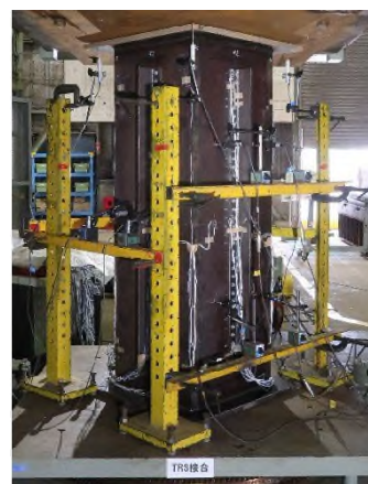
写真-2 座屈耐荷力試験 Photo-2 Buckling strength test
