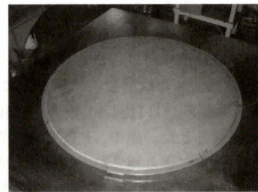
写真-5 新構造すべり板 Photo 5 Newly tested slide plate
