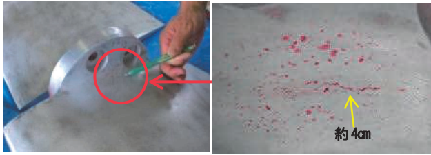
写真-4 動翼根元の欠陥(線状浸透指示模様) Photo 4 Small crack in fan blade(Penetrant testing)
