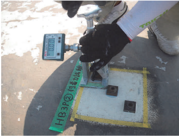
写真-1 既設塗膜の付着力試験 Adhesion test of existing coating
