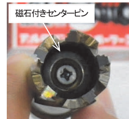
写真-10 Uリブ側削孔刃 Photo 10 Cutting blade for trough rib
