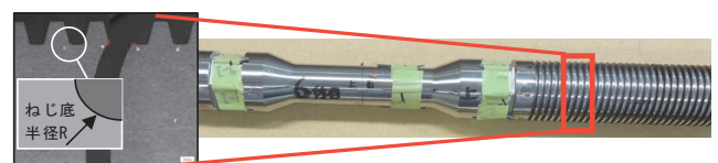
図-3 ねじ底半径Rの位置 Fig.3 Position of screw root radius R
