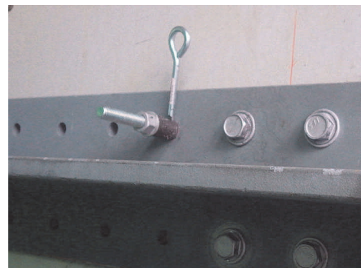
写真-9 引き寄せ治具 Photo 9 Jig for fixture
