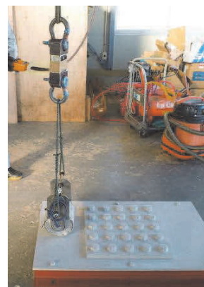
写真-3 磁石車輪の単体試験の状況 Photo 3 Situation of magnetic wheel unit test
